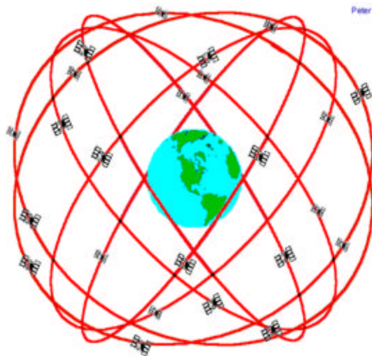
GPS Nominal Constellation 24 Satellites in 6 Orbital Planes 4 Satellites in each Plane 20,200 km Altitudes, 55 Degree Inclination
